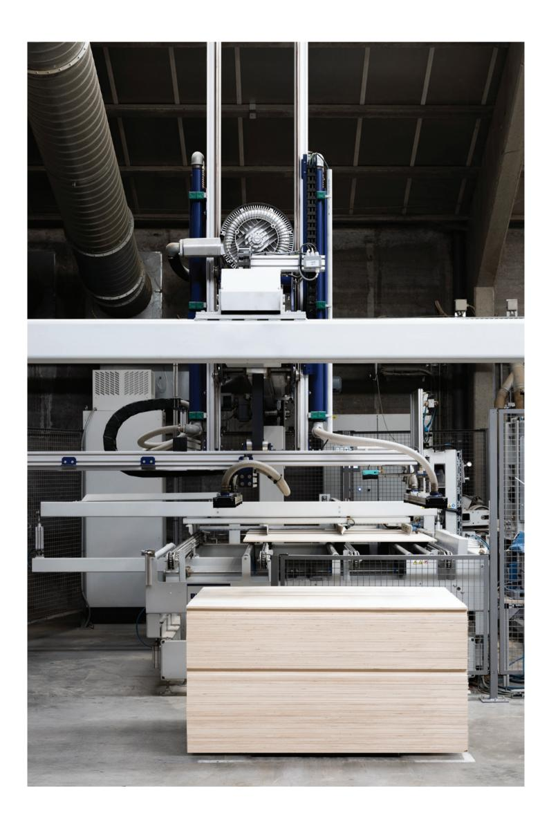
First, the sawn top layers are sorted by hand, after which they are glued to the plywood using a cold press technique. Belgiqa uses high-tech machines in the production process. This means we can guarantee a perfect fit. Afterwards, the boards are manually removed from the machines for an extra visual check. 011 🖪
