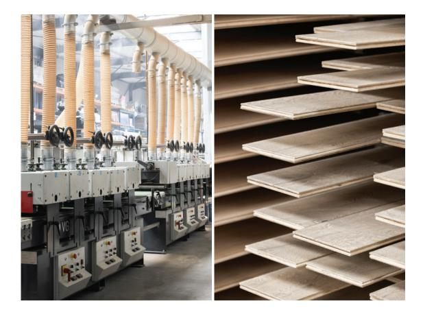
In a nutshell, that's what Belgiqa does day in, day out. The possibilities for parquet finishing are endless. Depending on the customer's preferences, the planks may or may not be brushed, sanded, aged, or treated with a band saw. Subsequently, if desired, they are stained, oiled, or varnished. In certain collections, multiple stains are layered, tannins are added, or the planks are bleached, resulting in a more profound colouring.
